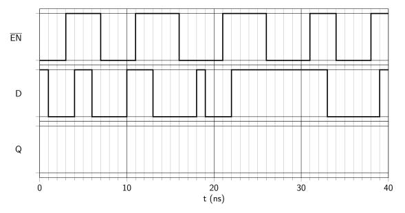
5. (10 points) Fill out the following timing diagram for a rising-edge triggered JK flip-flop. Ignore all gate delays. Q(0) = 1.
