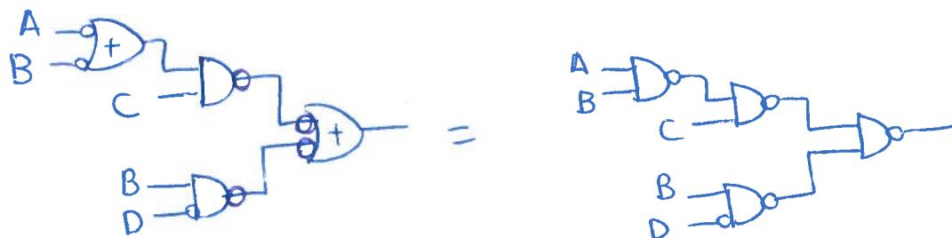
(i) (5 points) Draw the lowest cost circuit diagram as a NOR-only circuit. (Use either the double prime or bubble method and show your work.)
