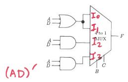
(a) (5 points) What is the MUX equation corresponding to the above circuit?
