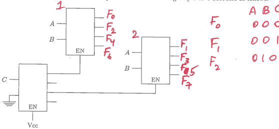
(a) (7 points) Label the above circuit diagram with outputs from  $F_0 - F_7$ .
