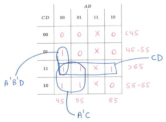
(b) (10 points) Use a k-map to solve for G, which indicates if the car is driving dangerously. All loops must be labeled to receive any credit.
