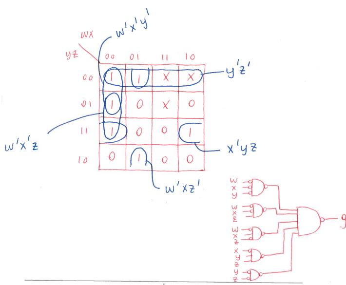
2. A sensor is capable of determining whether or not a car is speeding (driving faster than the speed limit) or driving dangerously (driving faster than 10 m.p.h. above the speed limit). The sensor receives the following codes. AB corresponds to the speed limit, and CD corresponds to the speed of the vehicle.
