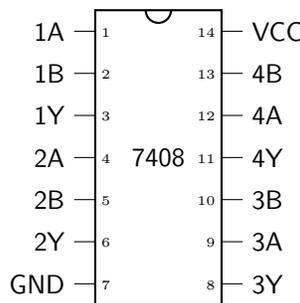
**Figure 2.2:** Pinout diagram of the 7408 chip.
