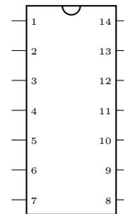
**Figure 2.1:** Diagram of a DIP chip with 14 pins.
